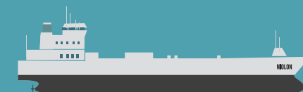
SEA-GOING RO-RO VESSEL - 967 LIN. M/80 SEMI-TRAILERS Used on the FerryMar (Caribbean inter-islands) service
